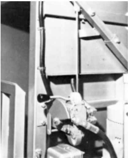
Fig. 6: Mechanical interlock (guard open)
